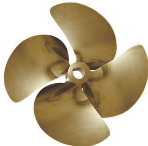
Dia 39"x Pitch 46"x 4 Blade, DAR 0.90% to obtain speed of 30 knots
