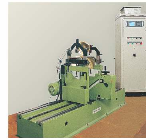
Dynamic Balancing up to Dia 1.5 Meter
