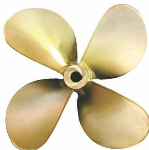
Dia 39"x Pitch 42"x 4 Blade, DAR 0.65% to obtain speed of 26 knots
